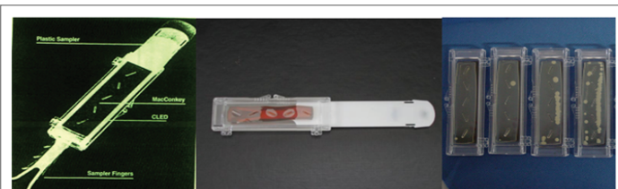
Figure 1: The original Diaslide device was a clinical tool for identification of urine bacterial colonies, hence consisted the MacConkey agar as medium.
